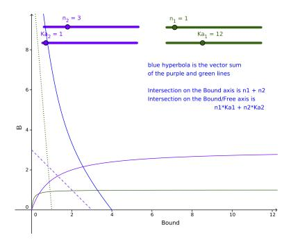
Figure 2.3 Example of a non-linear Scatchard plot with 2 classes of equivalent binding
